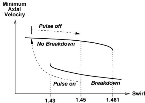
Figure 4: Schematic of the procedure for breakdown to no breakdown transition tests.
