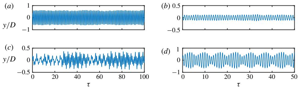
FIGURE 16. (Colour online) Time traces of the sphere displacement for  $f_R = 0.3$  (a,c) and  $f_R = 0.9$  (b,d) for a velocity ratio of  $\alpha_R = 1$ . (a,c) Time traces for  $U^* = 8$  and  $15$ , respectively. (b,d) Time traces for  $U^* = 6$  and  $U^* = 10$ , respectively.
