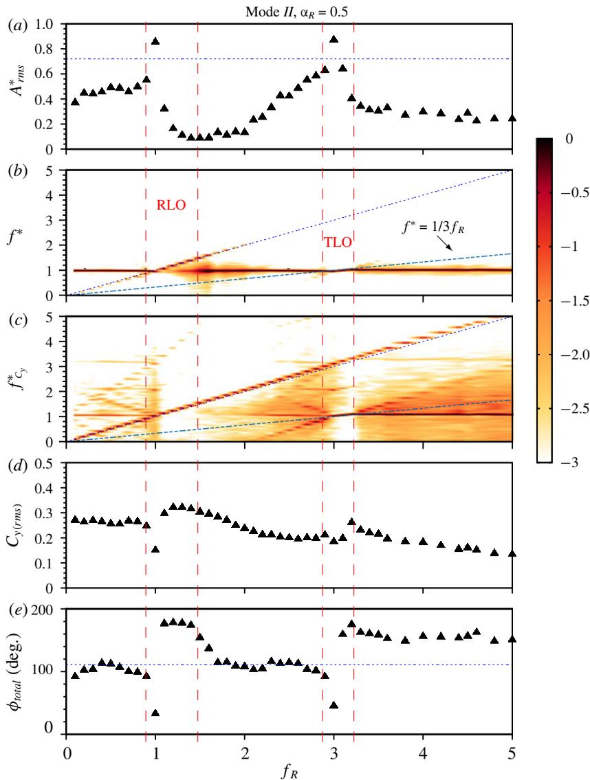
FIGURE 7. (Colour online) The response quantities of an elastically mounted sphere with imposed rotary oscillations is presented as a function of forcing frequency ratio,  $f_R$ , at a fixed velocity ratio of  $\alpha_R = 0.5$  in mode II ( $U^* = 10$ ). Refer to figure 4 for further details.
