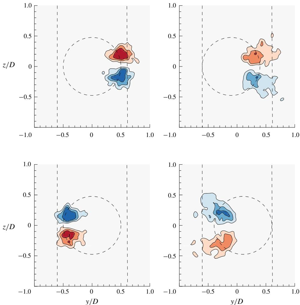
FIGURE 22. (Colour online) Streamwise vorticity plots showing the dominant counter-rotating vortex pair in mode I ( $U^* = 6$ ) for the frequency ratio of  $f_R = 0.9$  under lock-on. Refer to figure 21 for further details.
