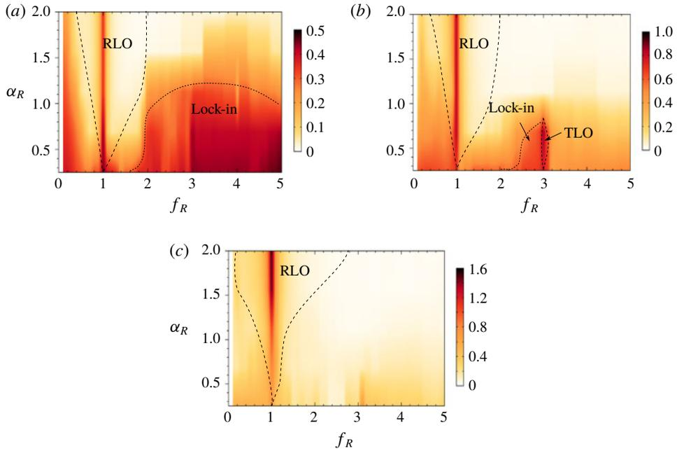
FIGURE 14. (Colour online) Plots showing the contours of  $A_{rms}^*$  as a function of  $\alpha_R$  and  $f_R$  in mode I (a), mode II (b) and mode III (c). Different regions highlighted with dashed lines.
