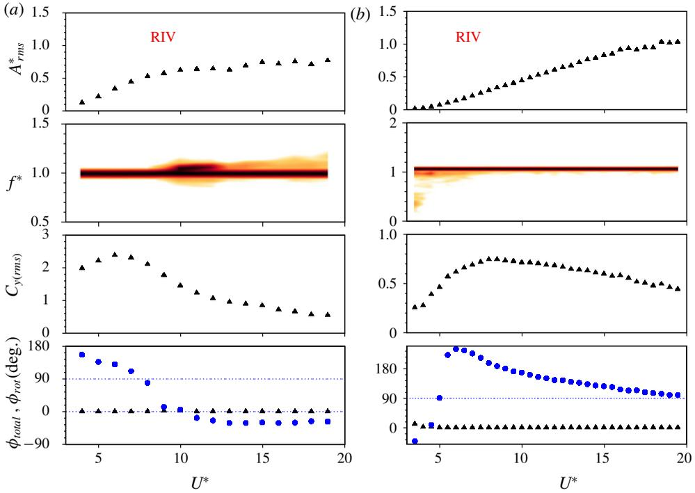
FIGURE 17. (Colour online) The response of an elastically mounted sphere with imposed rotary oscillations is presented as a function of reduced velocity for a fixed frequency ratio of  $f_R = 1.0$  (a) and  $f_R = 1.1$  (b) at a value of  $\alpha_R = 1$ . Refer to figure 4 for further details.
