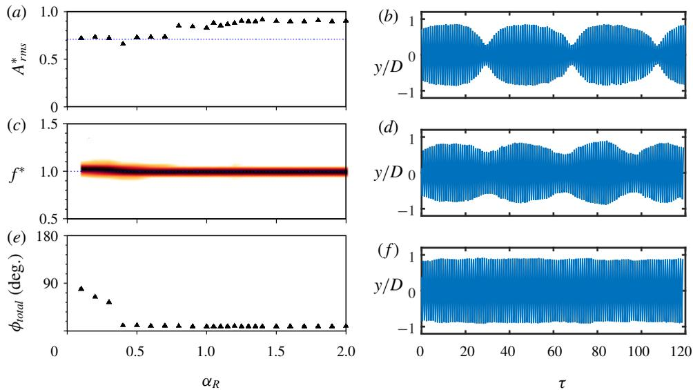
FIGURE 13. (Colour online) The response quantities of an elastically mounted sphere with the imposed rotary oscillations is presented as a function of velocity ratio,  $\alpha_R$ , at a fixed frequency ratio of  $f_R = 1$  (a,c,e) for mode II. (b,d,f) The time traces of the sphere displacement for  $\alpha_R = 0.3$  (b),  $\alpha_R = 0.6$  (d) and  $\alpha_R = 1.2$  (f).
