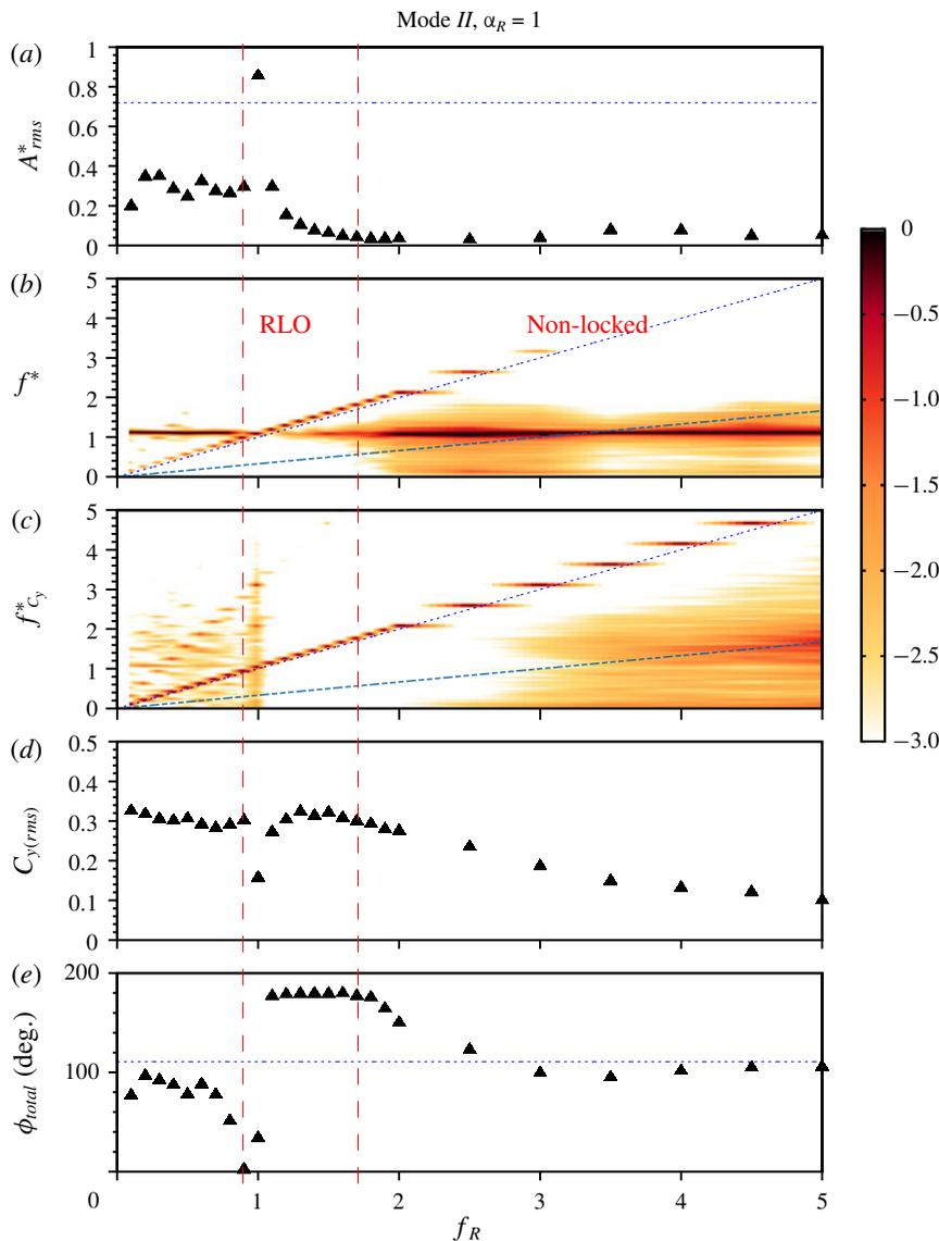
FIGURE 9. (Colour online) The response of an elastically mounted sphere with imposed rotary oscillations is presented as a function of forcing frequency ratio,  $f_R$ , at a fixed velocity ratio of  $\alpha_R = 1$  in mode II ( $U^* = 10$ ). Refer to figure 4 for further details.
