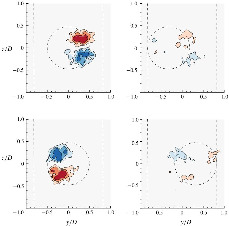
FIGURE 25. (Colour online) Streamwise vorticity plots showing the dominant counter-rotating vortex pair in mode I ( $U^* = 6$ ) for a frequency ratio of  $f_R = 1.0$  under resonance. Refer to figure 21 for further details.
