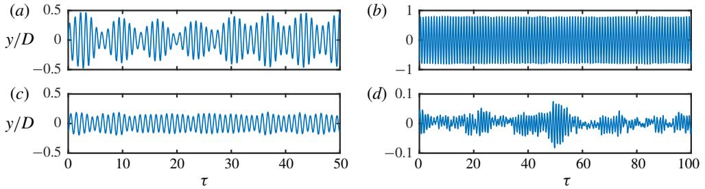
FIGURE 12. (Colour online) Time traces of the sphere displacement for frequency ratios  $f_R = 1.2$  (a,c) and  $f_R = 3$  (b,d) at two different velocity ratios of  $\alpha_R = 0.3$  and  $\alpha_R = 1.3$ .
