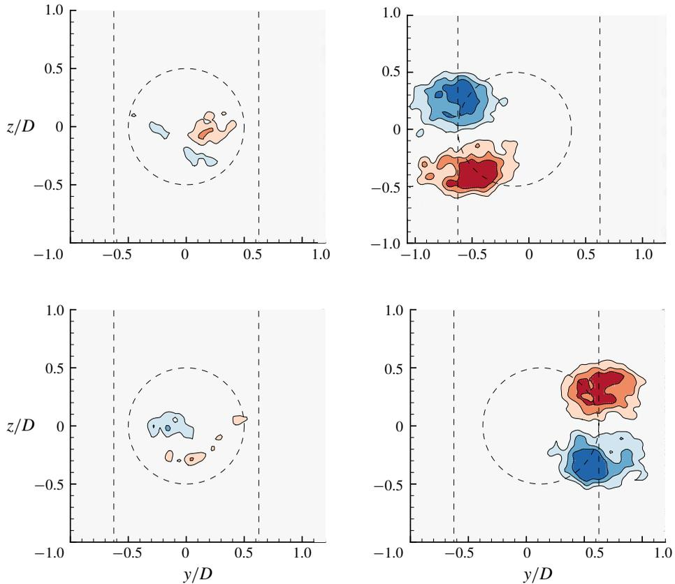
FIGURE 23. (Colour online) Streamwise vorticity plots showing the dominant counter-rotating vortex pair in mode I ( $U^* = 6$ ) for  $f_R = 1.1$  during the lock-on phenomenon. Refer to figure 21 for further details.
