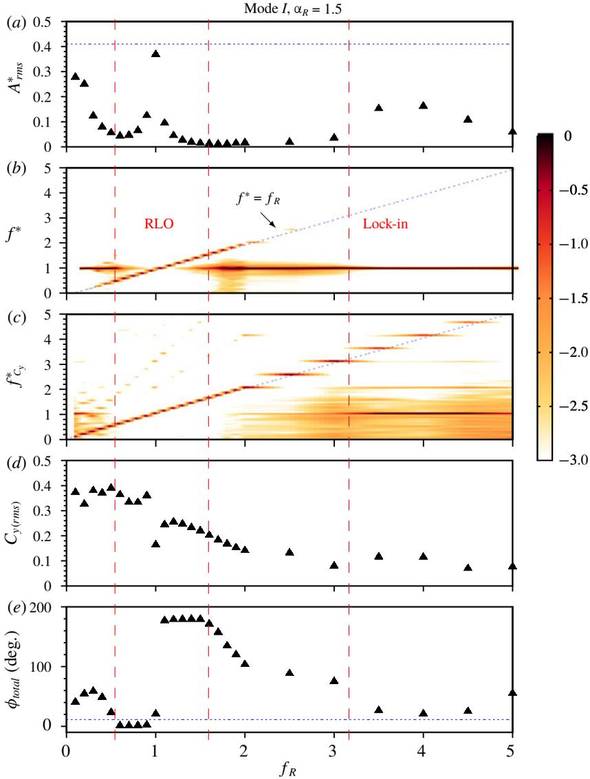
FIGURE 6. (Colour online) The response of an elastically mounted sphere under imposed rotary oscillation is presented as a function of forcing frequency ratio,  $f_R$ , at the fixed velocity ratio of  $\alpha_R = 1.5$  in the mode I region ( $U^* = 6$ ). Refer to figure 4 for further details.
