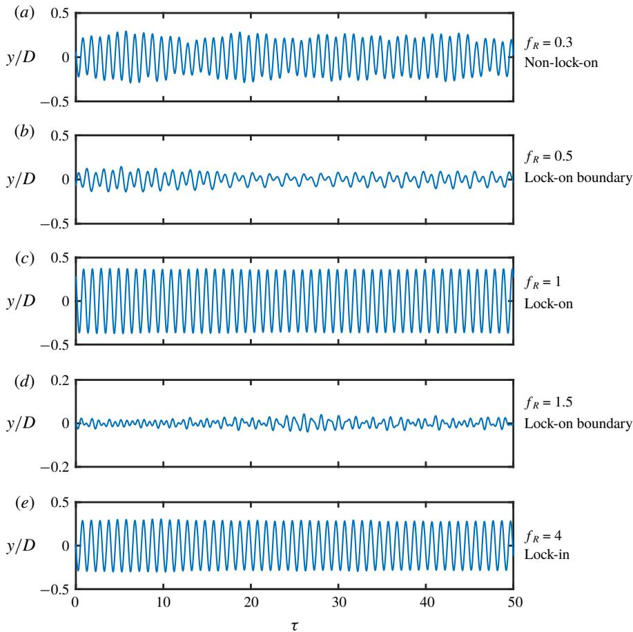
FIGURE 5. (Colour online) Time traces of the sphere displacement in mode I for different frequency ratios of (a)  $f_R = 0.3$ , (b)  $f_R = 0.5$ , (c)  $f_R = 1$ , (d)  $f_R = 1.9$  and (e)  $f_R = 4$ . The velocity ratio is fixed at  $\alpha_R = 1$ .
