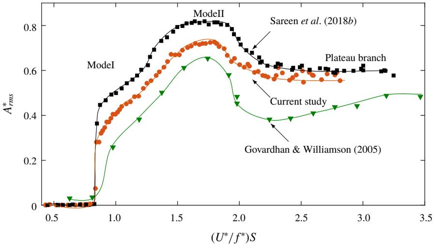
FIGURE 3. (Colour online) Amplitude response of an elastically mounted sphere (1-DOF) obtained in the current study (●) with a mass damping of  $(m^* + C_A)\zeta = 0.03$  compared to previous studies by Govardhan & Williamson (2005) (▼) with a mass damping approximately 0.92 and Sareen *et al.* (2018*b*) (■) with a mass damping of 0.0169.
