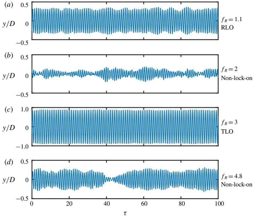
FIGURE 8. (Colour online) Time traces of the sphere displacement in mode II for different frequency ratios of (a)  $f_R = 1.1$ , (b)  $f_R = 2$ , (c)  $f_R = 3$  and (d)  $f_R = 4.8$ . The velocity ratio is fixed at  $\alpha_R = 0.5$ .
