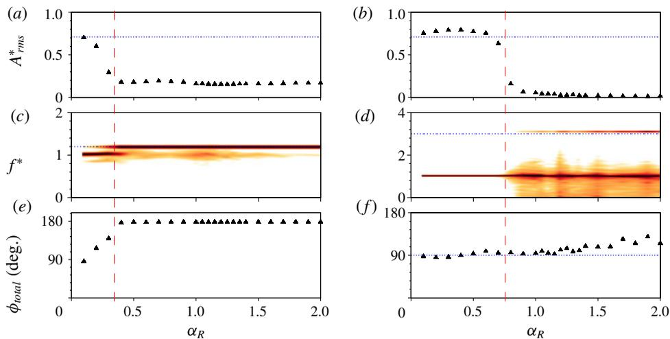
FIGURE 11. (Colour online) The response quantities of an elastically mounted sphere with imposed rotary oscillations is presented as a function of velocity ratio,  $\alpha_R$ , at fixed frequency ratios of  $f_R = 1.2$  (a,c,e) and  $f_R = 3$  (b,d,f) in mode II. The dashed red line demarcates the two regions obtained as the velocity ratio is varied in the above cases. The vibrations are greatly suppressed beyond the dashed line for both the frequency ratios shown above.
