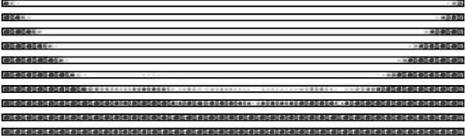
FIGURE 8. Development of Taylor-vortex flow after an instantaneous increase in Reynolds number from 70 to 116.67 as depicted by greyscale azimuthal vorticity. From top to bottom, the cross-sections correspond to non-dimensional times: t=0, 25, 50, 75, 100, 125, 150, 175, 250 and 500 . Fixed end conditions are used. The aspect ratio was \Gamma = 80.12 corresponding to 40 critical wavelengths.
