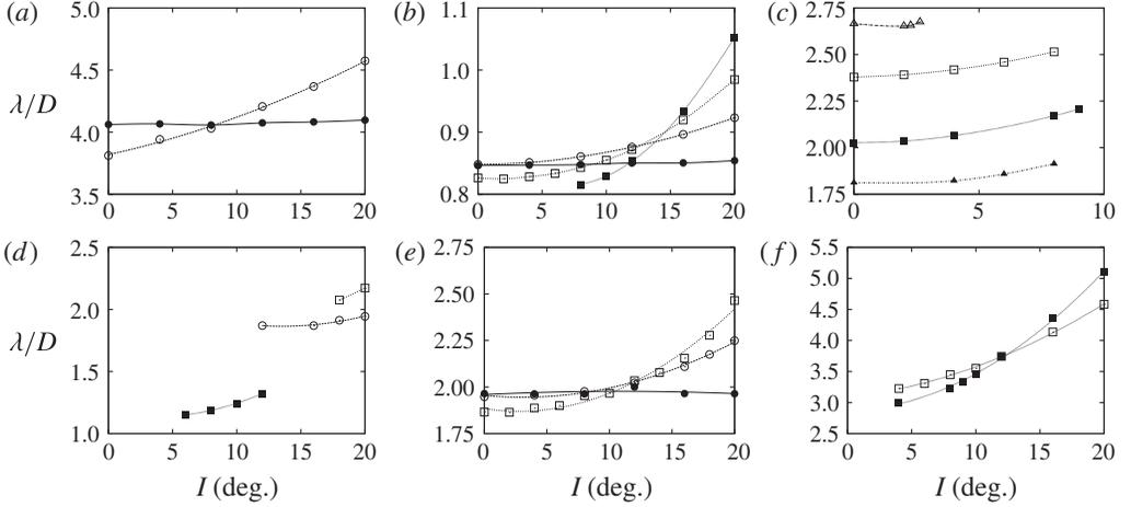
FIGURE 8. Variation of the critical spanwise wavelength at onset for  $Re \leq 500$  for (a) mode A, (b) mode B, (c) mode  $\hat{B}$ , (d) mode C, (e) mode QP and (f) mode QPA. The aspect ratios are assigned a specific symbol and line type;  $\Gamma = 1.1$  ( $\bullet$ ),  $\Gamma = 1.5$  ( $\circ$ ),  $\Gamma = 1.8$  ( $\triangle$ ),  $\Gamma = 2$  ( $\square$ ),  $\Gamma = 2.5$  ( $\blacksquare$ ) and  $\Gamma = 3$  ( $\blacktriangle$ ).
