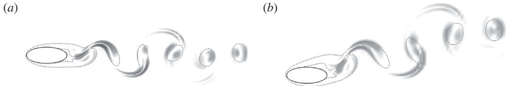
FIGURE 12. (Colour online) Visualisation of the spanwise perturbation vorticity contours in the wake of an elliptical cylinder of  $\Gamma = 2.5$  for (a)  $I = 0^\circ$ ,  $Re = 460$ ,  $\lambda/D = 3.6$  and (b)  $I = 16^\circ$ ,  $Re = 290$ ,  $\lambda/D = 4.5$ . Contour shading as per figure 6. Flow is from left to right in all images.
