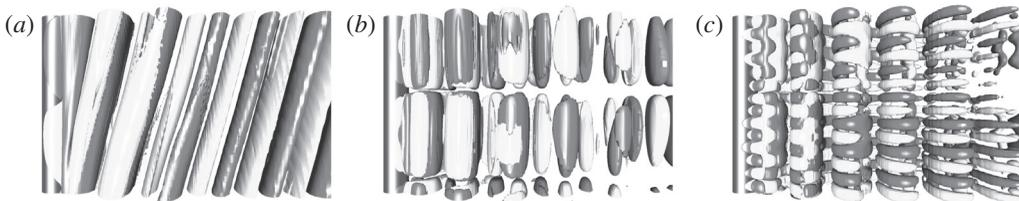
FIGURE 27. (Colour online) Visualisations of the streamwise vorticity (in red and yellow) in the wake of the elliptical cylinder (in blue) in plan view at  $\Gamma = 2.25, I = 0^\circ$  for a cylinder of spanwise distance of  $16D$ , at (a)  $Re = 300, \tau = 618$ , (b)  $Re = 320, \tau = 649$  and (c)  $Re = 320, \tau = 1079$ . Flow is from left to right in these images.
