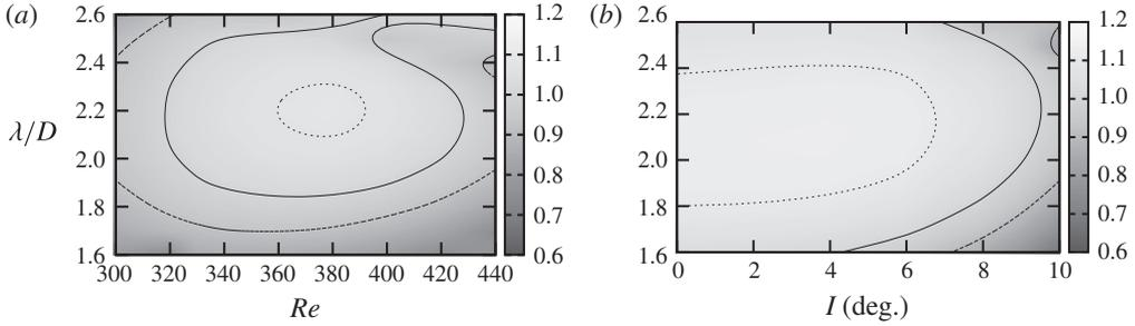
FIGURE 18. (Colour online) Contour plots of the Floquet multiplier of mode  $\hat{B}$  for  $\Gamma = 2.5$ : (a) as a  $f(Re, \lambda/D)$  at a constant incident angle of  $I = 8^\circ$  and (b) as a  $f(I, \lambda/D)$  at a constant Reynolds number of  $Re = 360$ . Contour lines in (a) are at  $|\mu| = 1.075$  (thin dashed lines), 1 (continuous line) and 0.925 (thick dashed lines). Contour lines in (b) are at  $\mu = 1.15$  (thin dashed lines), 1 (continuous line) and 0.9 (thick dashed lines).
