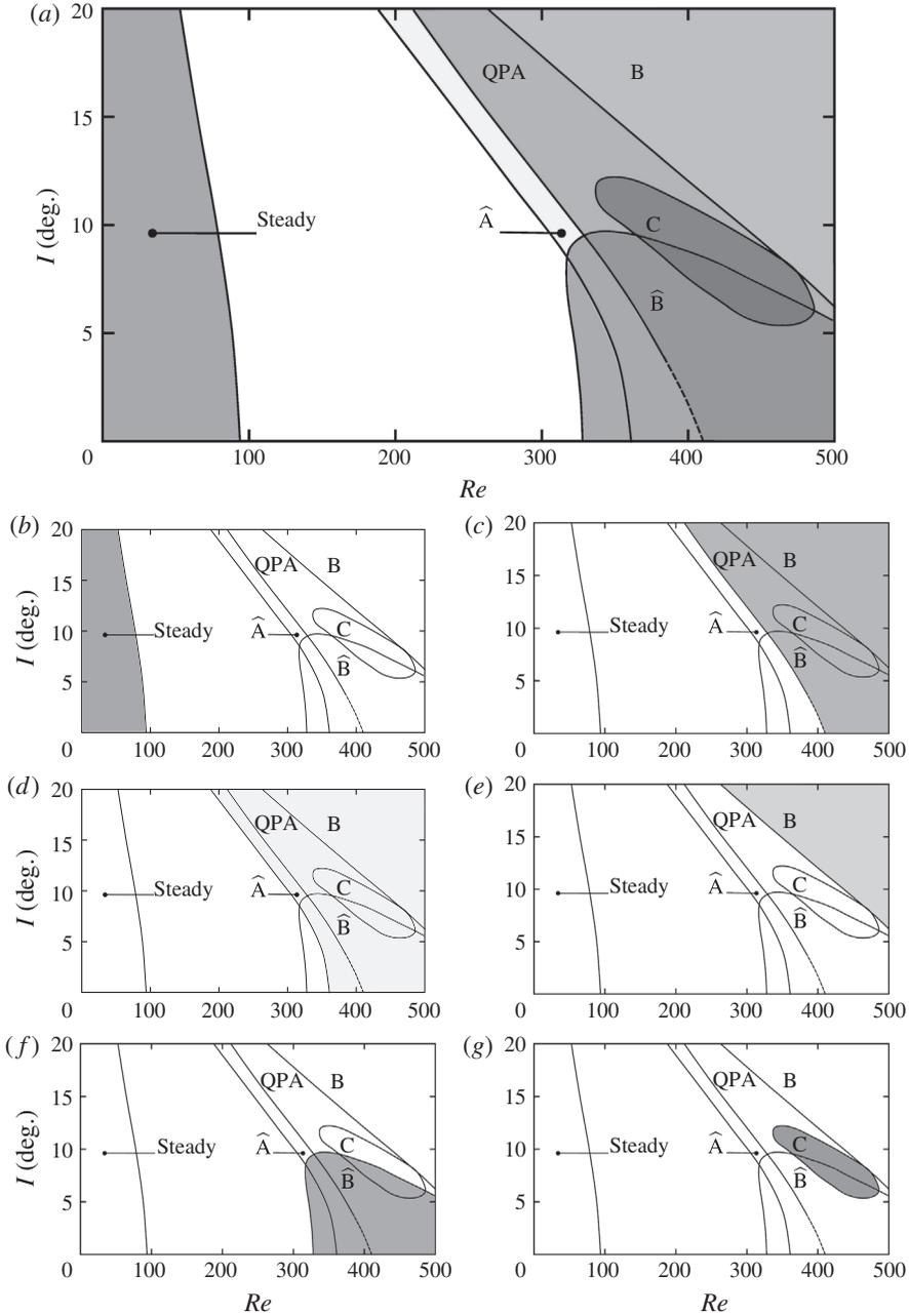
FIGURE 7. (Colour online) (a) Marginal stability diagram of the  $Re - I$  parameter space showing the various transitions for  $Re \leq 500, I \leq 20^\circ$  for the elliptical cylinder of  $\Gamma = 2.5$ . (b) Regions of steady flow and three-dimensional instabilities – (c) mode QPA, (d) mode  $\hat{A}$ , (e) mode B, (f) mode  $\hat{B}$  and (g) mode C are each assigned a unique colour and overlaying these regions gives the composite image in (a).
