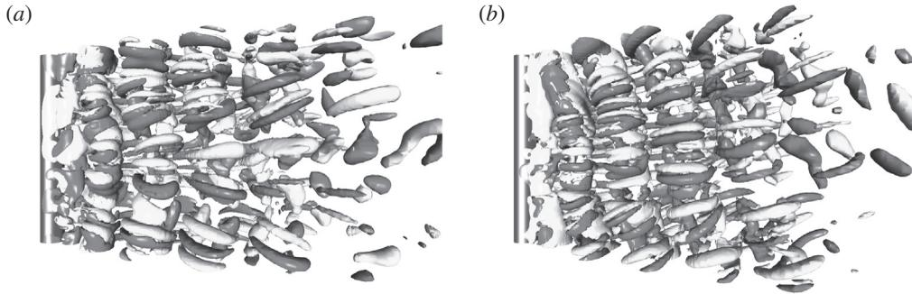
FIGURE 26. (Colour online) Visualisations of the streamwise vorticity (in red and yellow) in the wake of the elliptical cylinder (in blue) in plan view at  $\Gamma = 2, I = 12^\circ, Re = 320$  for a cylinder of spanwise distance of  $16D$ , at (a)  $\tau = 276$  and (b)  $\tau = 1903$ . Flow is from left to right in these images.
