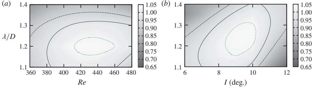
FIGURE 22. (Colour online) Contour plots of the Floquet multiplier of mode C for  $\Gamma = 2.5$ : (a) as a  $f(Re, \lambda/D)$  at a constant incident angle of  $I = 8^\circ$  and (b) as a  $f(I, \lambda/D)$  at a constant Reynolds number of  $Re = 400$ . Contour lines in (a b) are at  $|\mu| = 1.02$  (thin dashed lines), 0.96 (continuous line) and 0.9 (thick dashed lines).
