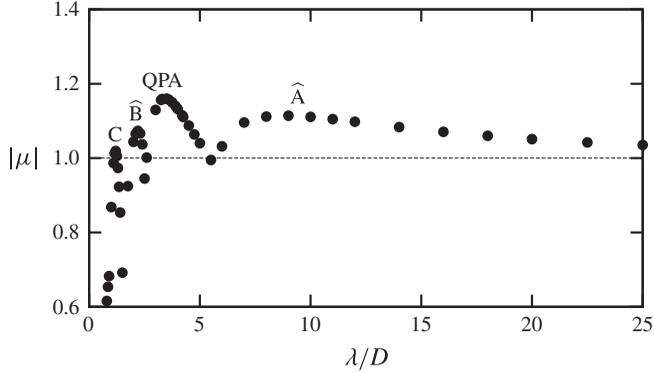
FIGURE 13. Variation of the Floquet multiplier with spanwise wavelength for the elliptical cylinder of  $\Gamma = 2.5$ , at  $I = 8^\circ$ ,  $Re = 400$ . The dashed line indicates neutral stability ( $|\mu| = 1$ ). The three-dimensional modes which are unstable – modes C,  $\hat{B}$ , QPA and  $\hat{A}$  are marked on this figure.
