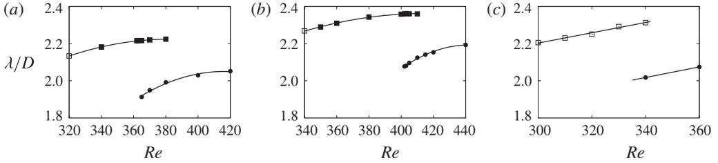
FIGURE 21. Variation of the dominant spanwise wavelength of mode C (●) and mode QP (□, ■) at  $I = 18^\circ$  for (a)  $\Gamma = 1.5$ , (b)  $\Gamma = 2$  and (c)  $\Gamma = 1.5$ ,  $I = 22^\circ$ . Open symbols indicate values when the mode is stable to perturbations ( $\mu < 1$ ), while filled symbols indicate values where Floquet multipliers are unstable ( $\mu \geq 1$ ). Lines are best fits to the measured values.
