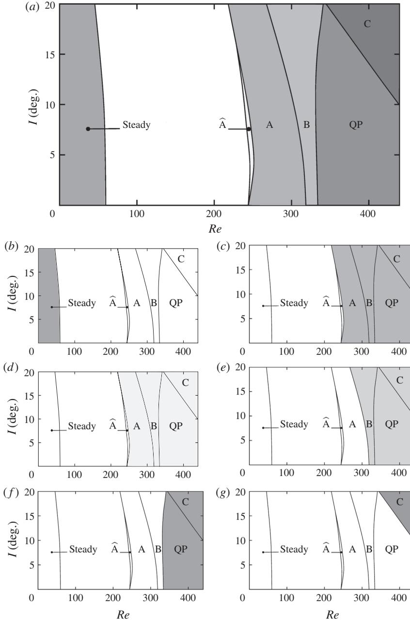
FIGURE 4. (Colour online) (a) Marginal stability diagram of the  $Re - I$  parameter space showing the various transitions for  $Re \leq 440, I \leq 20^\circ$  for the elliptical cylinder of  $\Gamma = 1.5$ . (b) Regions of steady flow and three-dimensional instabilities – (c) mode A, (d) mode  $\hat{A}$ , (e) mode B, (f) mode QP and (g) mode C are each assigned a unique colour and overlaying these regions gives the composite image in (a).
