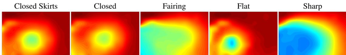
Figure 11: Stream-wise total pressure fields  $X = 1W, \psi = 15^\circ$ . Total pressure grid is fixed in tunnel aligned coordinates. Colour scale is the same as figure 10.
