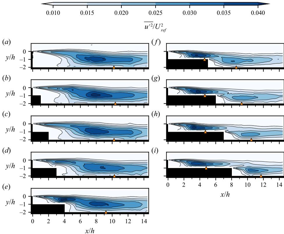
Figure 11. Normalised streamwise component of Reynolds stress ( $\overline{u'^2}/U_{ref}^2$ ) for:  $d = 0h$  (a);  $d = 1h$  (b);  $d = 2h$  (c);  $d = 3h$  (d);  $d = 4h$  (e);  $d = 5h$  (f);  $d = 6h$  (g);  $d = 7h$  (h);  $d = 8h$  (i). The  $\Delta$  (orange) markers indicate the mean reattachment location on the first (if applicable) and second steps.
