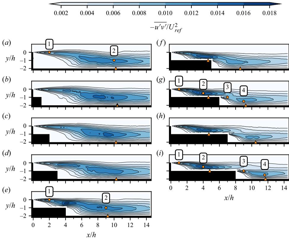
Figure 12. Normalised shear stress component of Reynolds stress ( $-\overline{u'v'}/U_{ref}^2$ ) for:  $d = 0h$  (a);  $d = 1h$  (b);  $d = 2h$  (c);  $d = 3h$  (d);  $d = 4h$  (e);  $d = 5h$  (f);  $d = 6h$  (g);  $d = 7h$  (h);  $d = 8h$  (i). The  $\Delta$  (orange) markers indicate the mean reattachment location on the first (if applicable) and second steps. The  $\circ$  (orange) markers indicate the locations used for power spectral density plots in figure 14.
