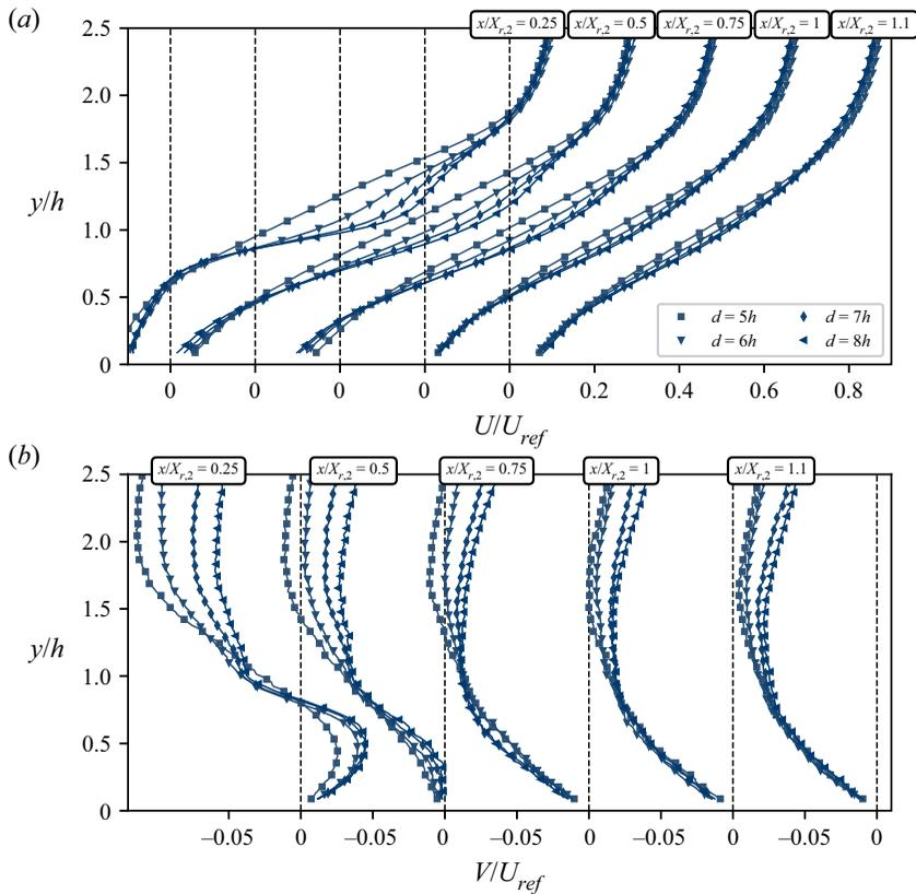
Figure 9. Mean streamwise (a) and y-direction (b) velocity profiles on the second step. Only the results for step separations where the flow reattaches on both steps are shown. The markers show every eighth PIV measurement location, for clarity.
