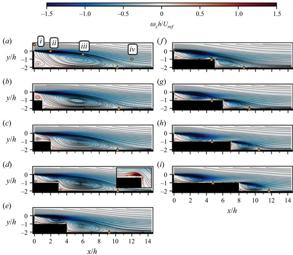
Figure 2. Streamlines of mean velocity and colour contours of out-of-plane vorticity ( $\omega_z$ ) for:  $d = 0h$  (a);  $d = 1h$  (b);  $d = 2h$  (c);  $d = 3h$  (d);  $d = 4h$  (e);  $d = 5h$  (f);  $d = 6h$  (g);  $d = 7h$  (h);  $d = 8h$  (i). The  $\Delta$  (orange) markers indicate the mean reattachment location on the first (if applicable) and second steps. The orange circle markers in (a) relate to table 1.
