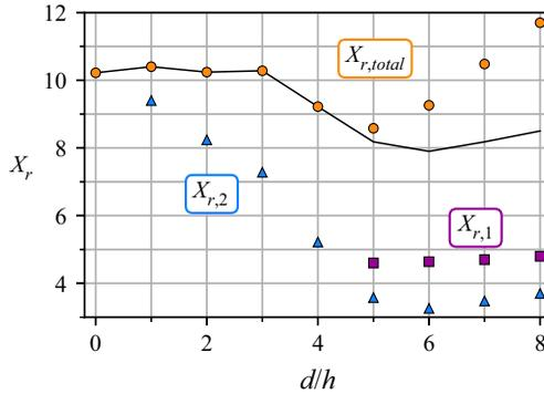
Figure 3. Reattachment length on the first step ( $X_{r,1}$ ), second step ( $X_{r,2}$ ), and the total reattachment length ( $X_{r,total}$ ) for varying step separation. The black line indicates the combined length of detached flow (i.e.  $X_{r,total}$  when the flow does not reattach on the first step, and  $X_{r,1} + X_{r,2}$  when the flow does reattach on the first step).
