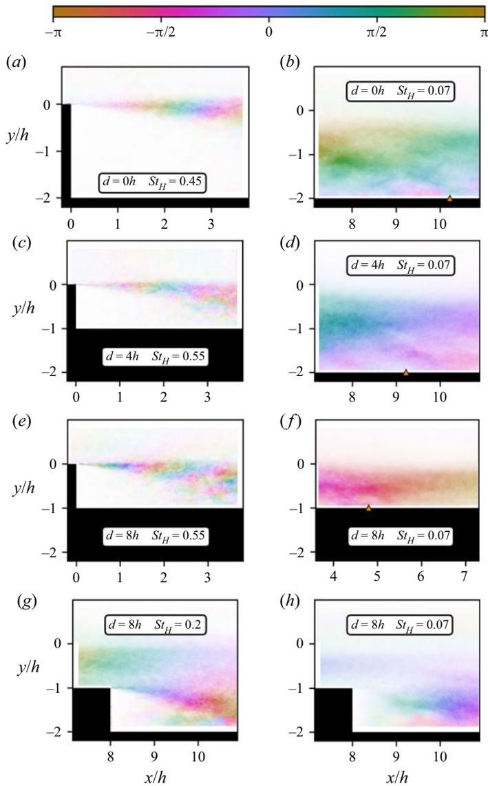
Figure 16. Phase map of the first SPOD mode for step separations and frequencies listed in each plot. The transparency of each plot is proportional to the spectral power of the first mode.
