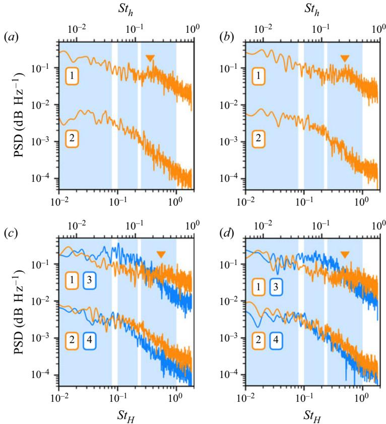
Figure 14. PSD estimates of the streamwise velocity for step separations of  $d = 0h$  (a),  $d = 4h$  (b),  $d = 6h$  (c) and  $d = 8h$  (d) at the three locations shown figure 12. Each PSD estimate is separated by two decades. The blue bands indicate regions over which the average power was plotted across the spatial domain in figure 15.
