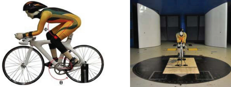
Fig. 1. Mannequin position/equipment and wind tunnel test-set up for both force and flow visualization studies
