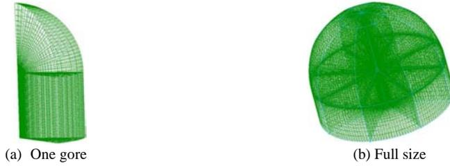
Fig. 2. The hemispherical parachute calculation grid.
