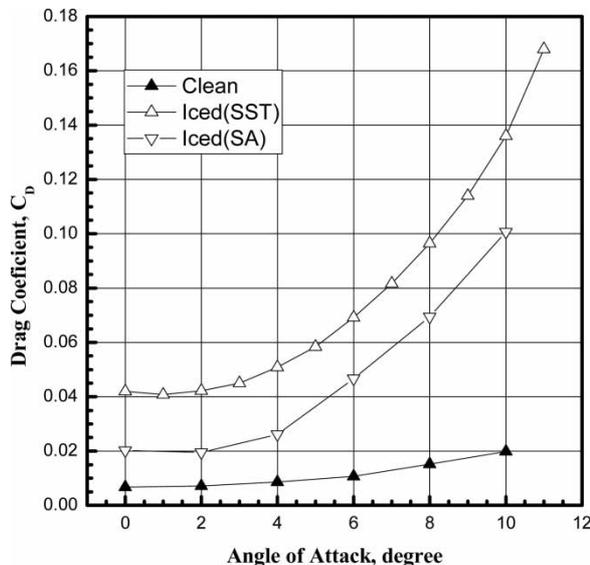
Fig. 4 Drag coefficient of B757/767 aerofoil with 145-m ice
