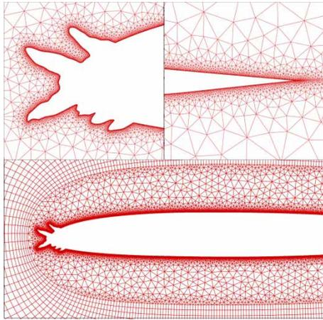
**Fig. 2** Hybrid grids on B757/767 aerofoil with 145-m ice
