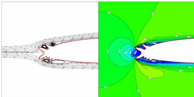
**Fig. 6** Mach contour and streamlines of 145-m iced aerofoil at  $AOA = 0^\circ$
