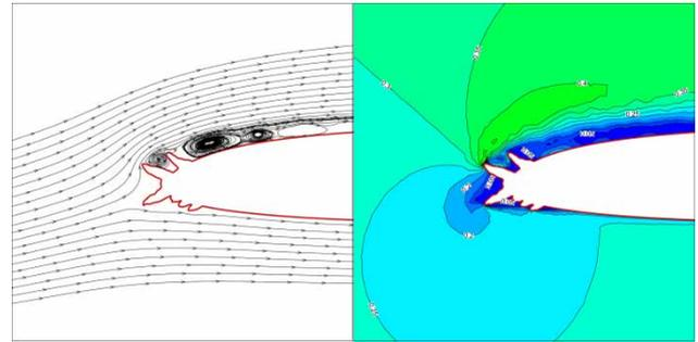
**Fig. 8** Mach contour and streamlines of 145-m iced aerofoil at  $AOA = 6^\circ$
