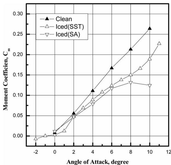
Fig. 5 Moment coefficient of B757/767 aerofoil with 145-m ice
