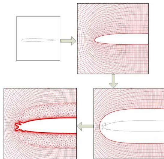
**Fig. 1** The process of generating a hybrid grid on complex iced aerofoil
