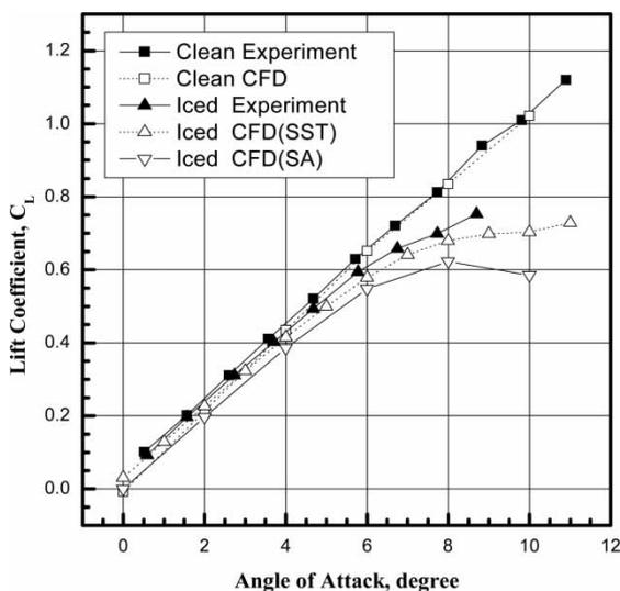
Fig. 3 Lift coefficient of B757/767 aerofoil with 145-m ice
