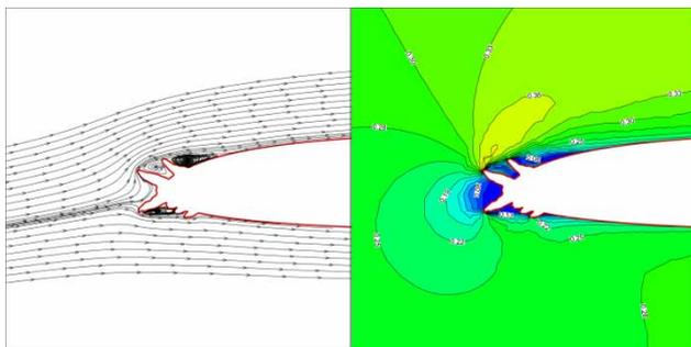
**Fig. 7** Mach contour and streamlines of 145-m iced aerofoil at  $AOA = 4^\circ$
