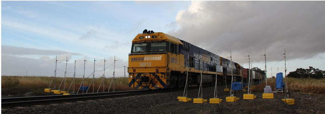
Figure 1: An operational full-scale inter-modal freight train driving past measurement rakes of 4-hole dynamic pressure probes, placed either side of the train.
