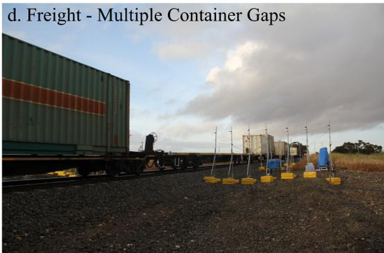
Figure 3: Variety of gap sizes between shipping containers observed on the different operational freight trains.
