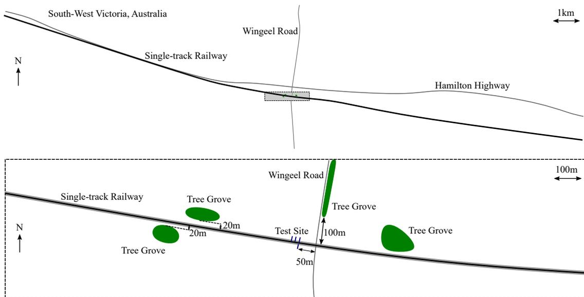
Figure 2: The experiment test site at Wingeel, Victoria, Australia. A large-scale view of the track and roads are illustrated (top), with the local topography and location of trees and vegetation illustrated in the zoomed-in figure inset below.
