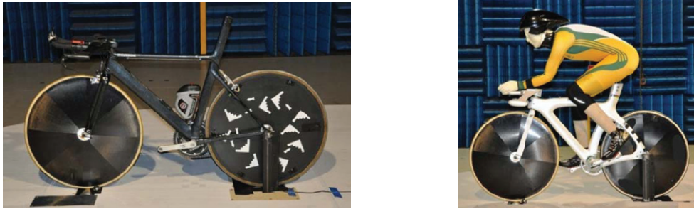
Fig. 2. (a) bicycle as used for bicycle only testing; (b) bicycle and mannequin setup
