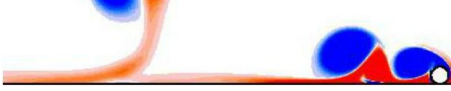
Figure 3: Process of vortex formation and shedding in the wake of the cylinder as the Reynolds number increases.
