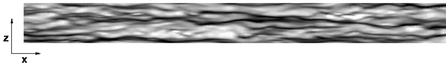
Figure 4. Instantaneous longitudinal velocity fluctuations in a wall-parallel plane at y^+ \approx 10 .
