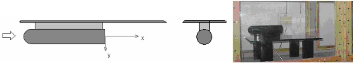
Figure 1. Schematic of test model and picture of its mounting arrangement in the wind tunnel.
