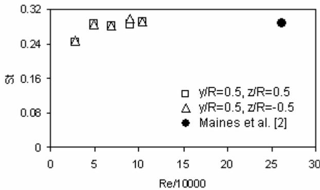
Figure 6. Wake Strouhal number obtained at  $x/D=2$ .
