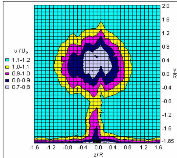
Figure 3. Velocity distribution in transverse (yz) plane at  $x/D=2$ .
