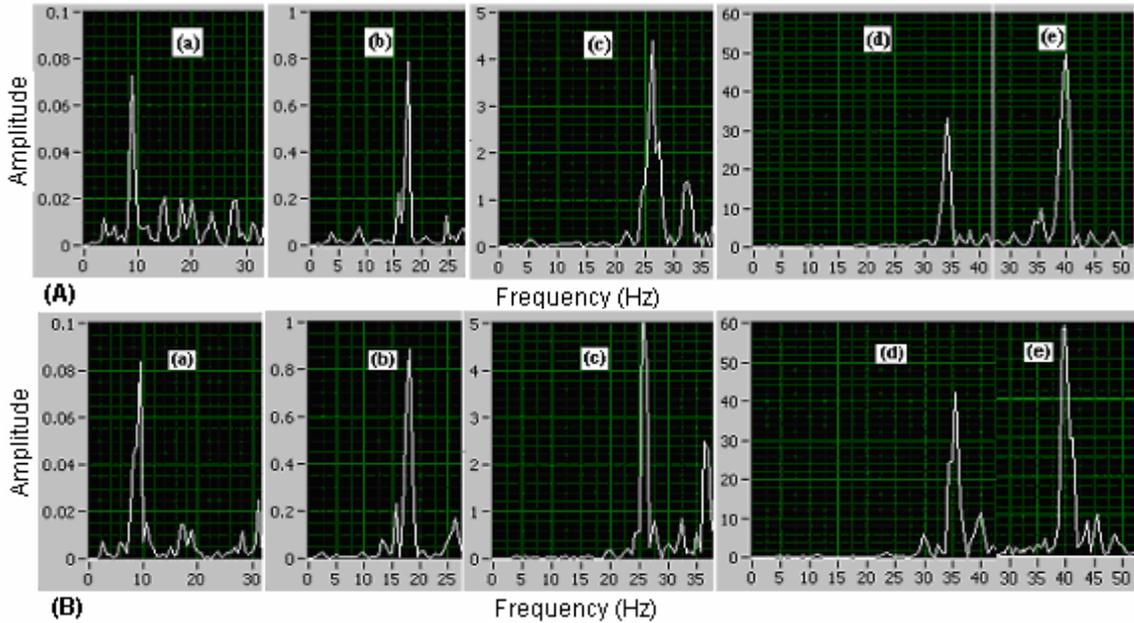
Figure 5. Frequency spectra in the first quadrant (A)  $y/R=0.5$ ,  $z/R=0.5$  and the second quadrant (B)  $y/R=0.5$ ,  $z/R=-0.5$  of the wake at  $x/D=2$  for different flow velocities. (a)  $U=4$  m/s, (b)  $U=7$  m/s, (c)  $U=10$  m/s, (d)  $U=13$  m/s and (e)  $U=15$  m/s.
