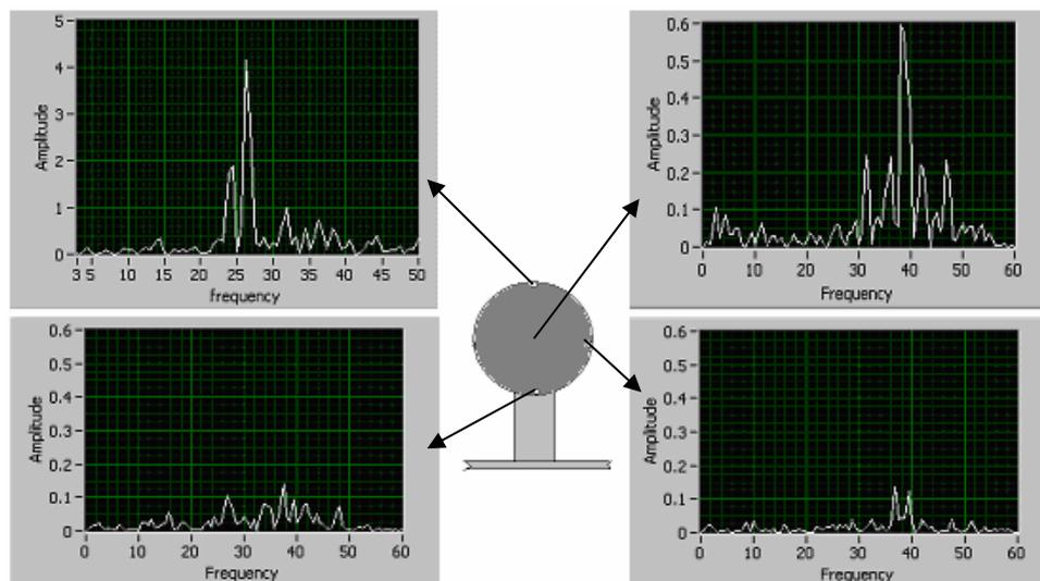
Figure 4. Frequency spectra of unsteady pitot pressures at various locations in the transverse yz plane at  $x/D=2$ .
