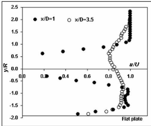
Figure 2. Velocity profiles in vertical (xy) plane at  $z/R=0$ .
