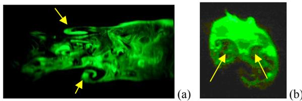
Figure 8. Wake flow visualization using smoke and laser sheet technique: (a) cut view in horizontal  $xz$  plane at  $y/R=0$ , (b) cut view in transverse  $yz$  plane at  $x/D=2$ .
