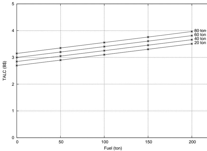
Figure 2: TALC as a function of  $W_{fuel}$ , for  $W_{wing} = 20, 40, 60, 80$  ton.
