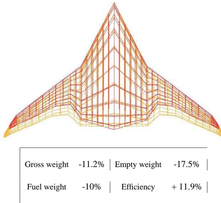
Figure 3: Comparison between optimized (dark) configuration and initial configuration
