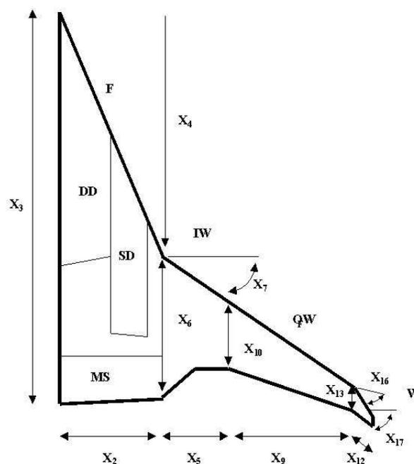
Figure 1: Sketch of the BWB model (F = Fuselage, IW = Inner Wing, OW = Outer Wing, W = Winglet, DD= Double Deck, SD = Single Deck, MS = Movable surface)
