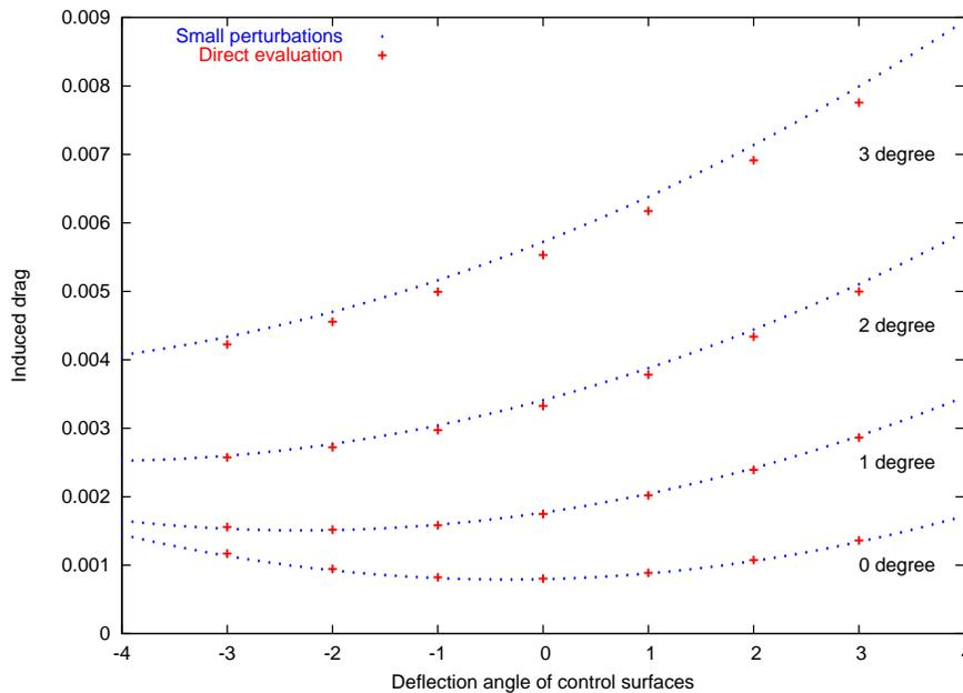
Figure 2: Comparison between direct evaluation of the induced drag and the small perturbation method for different angles of attack.
