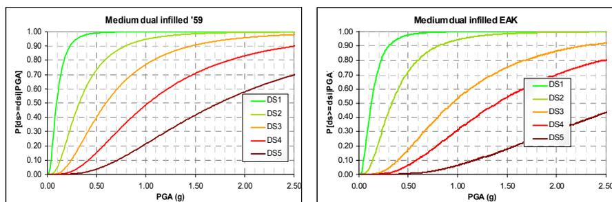
**Fig. 6** Fragility curves for medium-rise dual infilled systems, low (left) and high code design.
