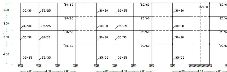
**Fig. 1** 4-storey building with dual system (bare structure)
