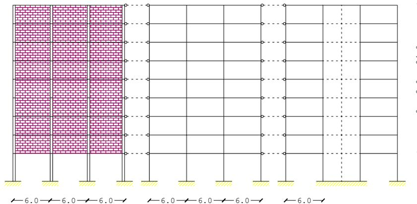
**Fig. 2** 9-storey building with dual system and pilotis
