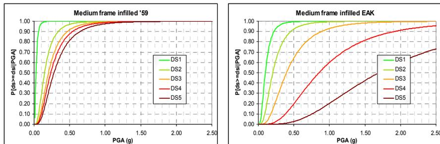
**Fig. 5** Fragility curves for medium-rise infilled frames, low (left) and high code design.
