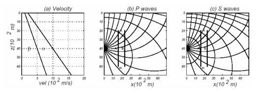
Figure 2.- Properties in a heterogeneous medium a) velocities  $\alpha(0) = 200m/s$ ,  $\beta(0) = 100m/s$ ,  $\rho(0) = 1T/m^3$  and h = 1000 m, b) and c) rays and wave fronts every 3 s. Set of stations A and B in thick line.
