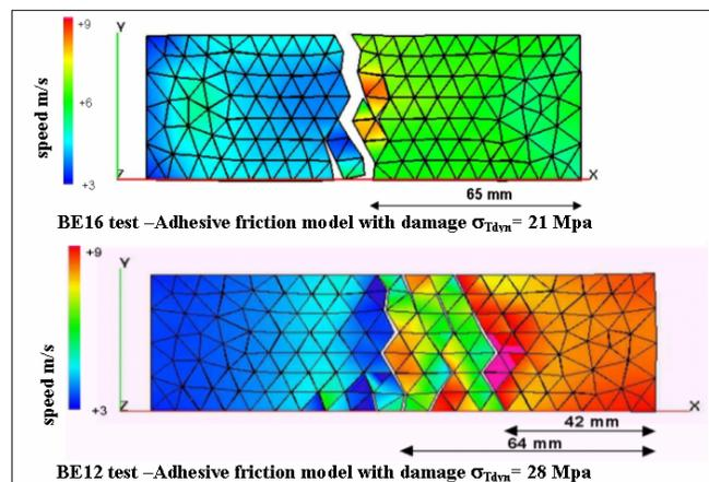
Figure 6: Rupture and axial velocity isovalues for BE16 and BE12 tests
