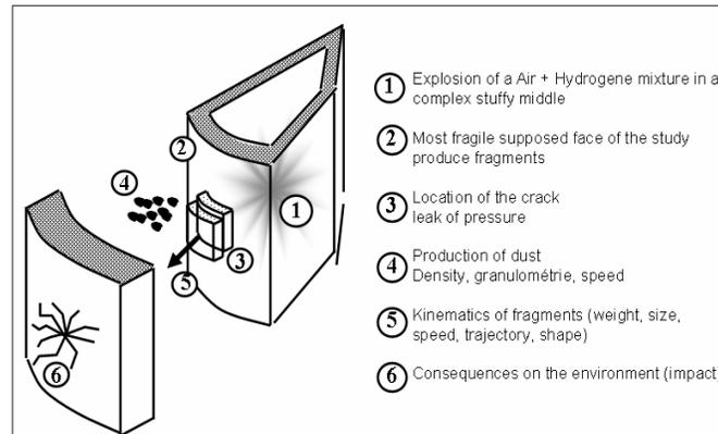
Figure 1: Accident scenario mechanisms
