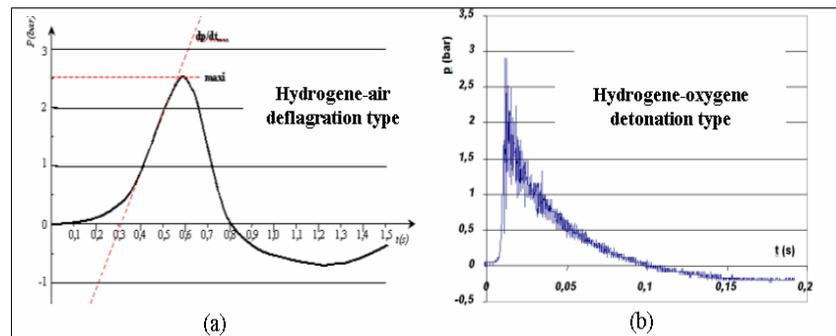
Figure 2: Pressure/time signals for a stuffy deflagration type (a) and a stuffy detonation type (b)
