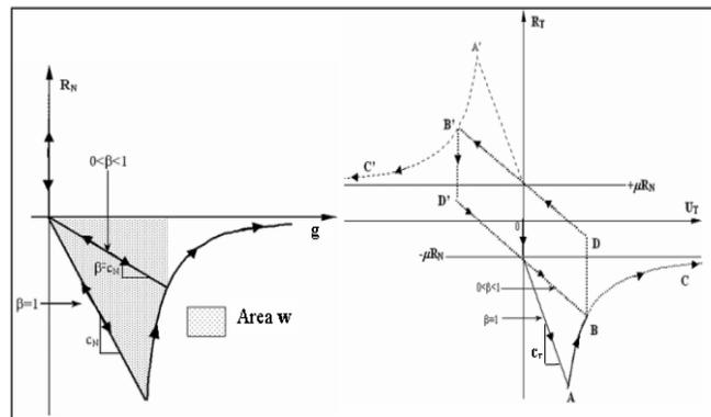
Figure 4: Cangémi-Fremond model – charge/discharge cycle for normal and tangential load
