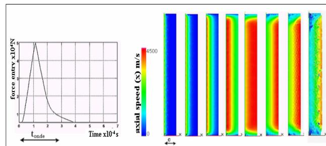
Figure 7: Wave transmission in a concrete wall and scaling
