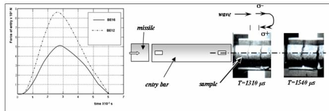
**Figure 5:** Modified Split Hopkinson Pressure Bar test - Incidental pressure signal– BE12 test with two high tension failure
