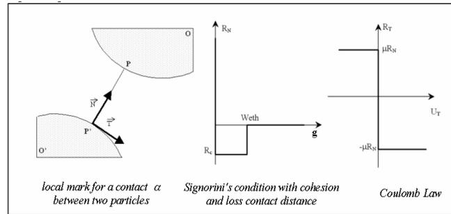
Figure 3: Normal cohesive model with fracture energy and coulomb law
