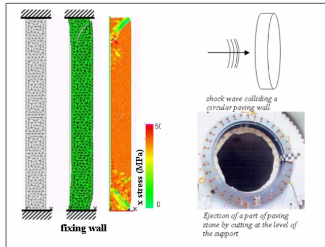
**Figure 8:** Bending of concrete wall and support condition influences. Slab ejection by shear failure on a shock tube test
