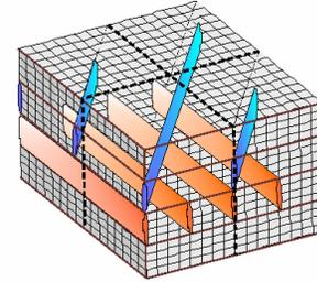
Figure 2: Transverse matrix cracks in a composite
