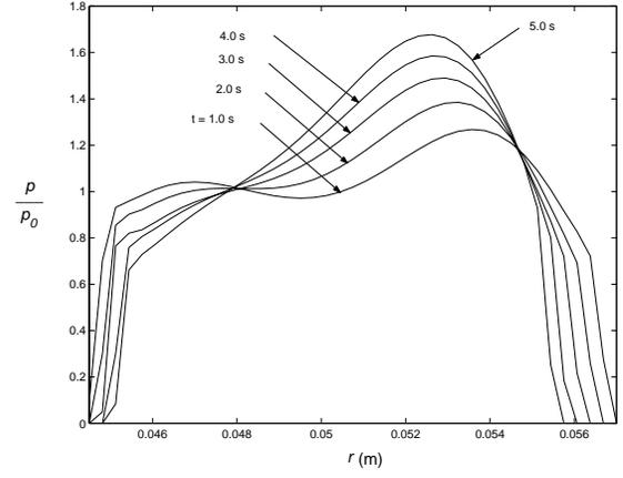
Figures (4, 5) Contact pressure distribution at different instants of time for  $\omega(0) = 0.75 \omega_c$
