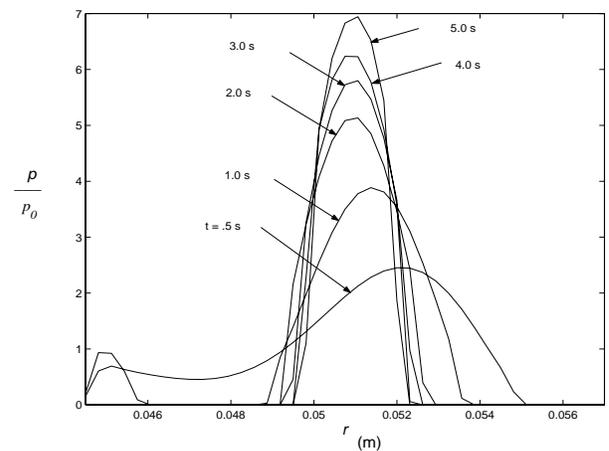
Figures (2, 3) Contact pressure distribution at different instants of time for  $\omega(0) = 1.5 \omega_c$
