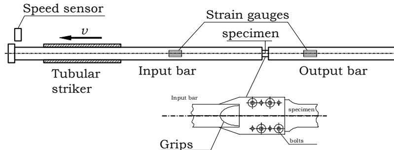
Figure 2: Schematic representation of the experimental set-up for tensile tests and detail of the grips for laminate specimens.
