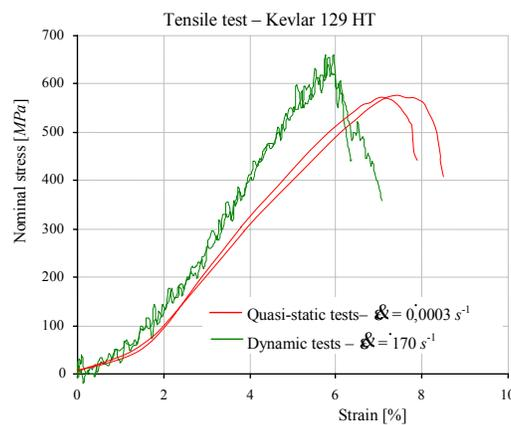
Figure 5: Comparison of stress-strain curves in quasi-static and dynamic condition
