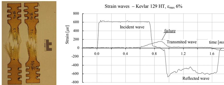
Figure 4: Geometry of a Kevlar® 129 HT specimen after test and recorded signals.
