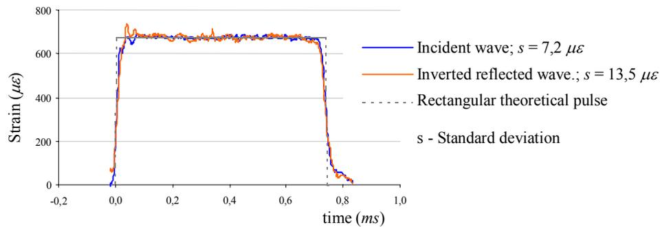
Figure 3: Comparison between incident and symmetric reflected waves.
