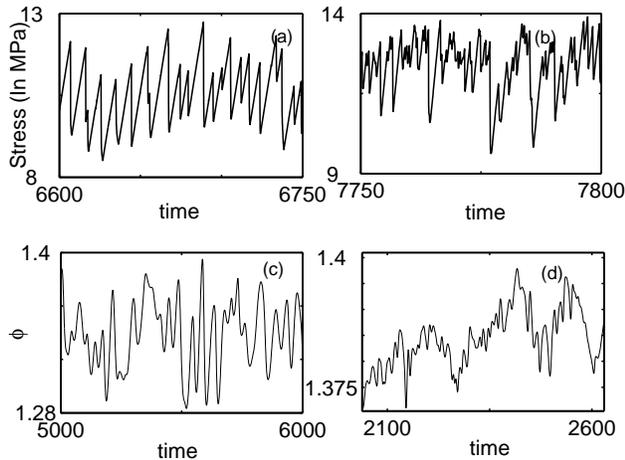
**Figure 1** : (a,b) Experimental stress-time series for the chaotic state at  $\dot{\epsilon}_a = 1.7 \times 10^{-5} s^{-1}$  and power law state at  $\dot{\epsilon}_a = 8.3 \times 10^{-5} s^{-1}$ . (c, d) Stress-time series from the model at  $\dot{\epsilon} = 120$  and  $\dot{\epsilon} = 280$  respectively.
