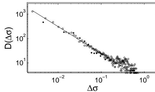
**Figure 3 :** Distributions of the stress drops from the model (o), from experiments (•) for  $N = 1000$  and  $\dot{\epsilon} = 280$ . Solid line is a guide to the eye.
