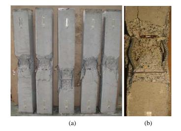
Figure 2: Experiments: (a) Series N10 after collapse. (b) Front view on the damaged zone at the midheight.
