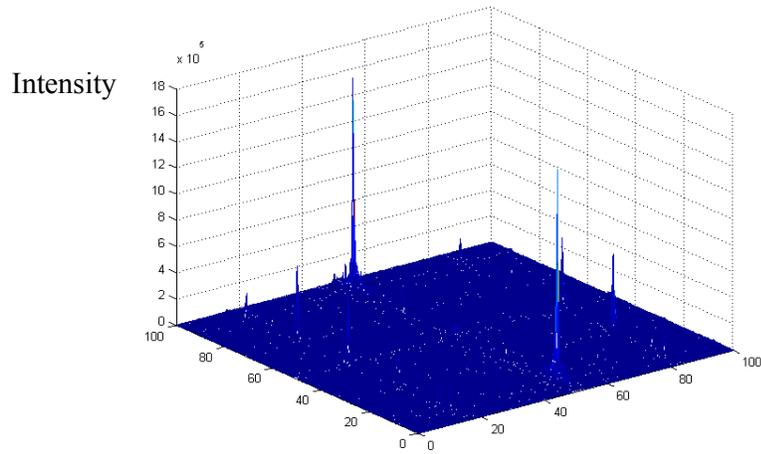
Fig. 1 Typical two dimensional power spectrum of the open-end sample.
