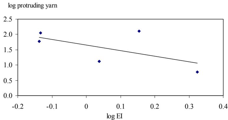
**Fig. 3** Variation of log protruding yarn VS log EI, R= -0.61, b= -1.8, a=1.65
