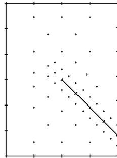
Figure 2: Dual boundary element mesh.
