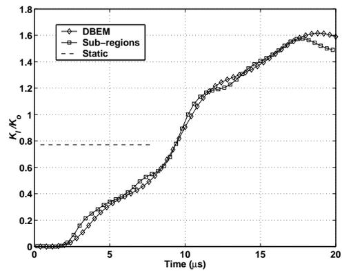
Figure 4: Normalised mode I dynamic stress intensity factors.
