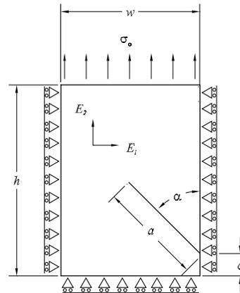
Figure 1: Plate with a slanted edge crack.
