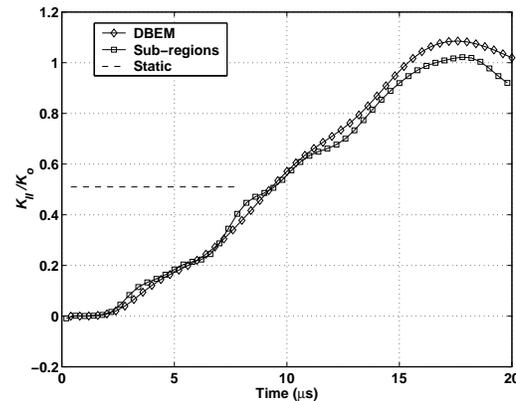
Figure 5: Normalised mode II dynamic stress intensity factors.
