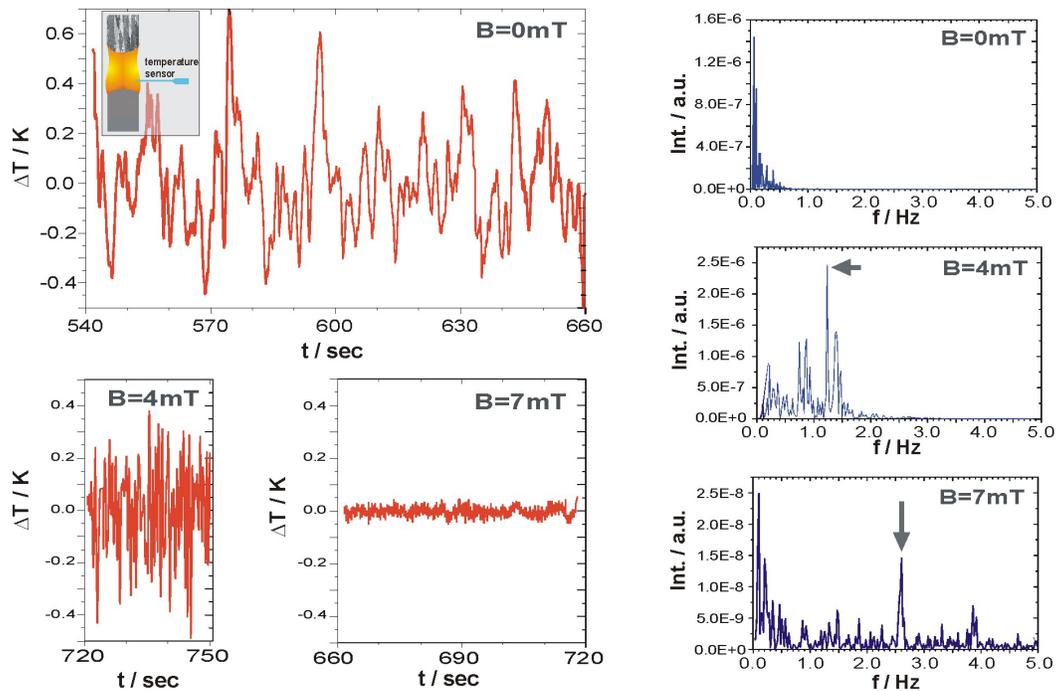
Fig. 3: Performing temperature measurements in the silicon melt (melt diameter: 10 mm), the three-dimensional, time-dependent character of the flow field becomes obvious. The flow instabilities are strongly reduced under the influence of a rotating magnetic field.
