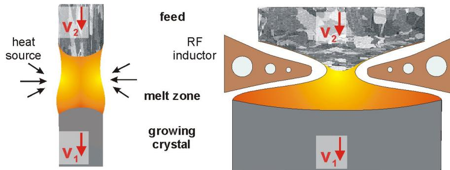
Fig. 1: Basic concept of the float zone process, on the left hand side for a conventional set-up heated by radiation or conduction and on the right hand side for the “needle-eye” technique. The growing crystal moves downward relative to the heater with a velocity  $v_1$ , which is in most cases independently controllable from the velocity  $v_2$  of the feed rod.
