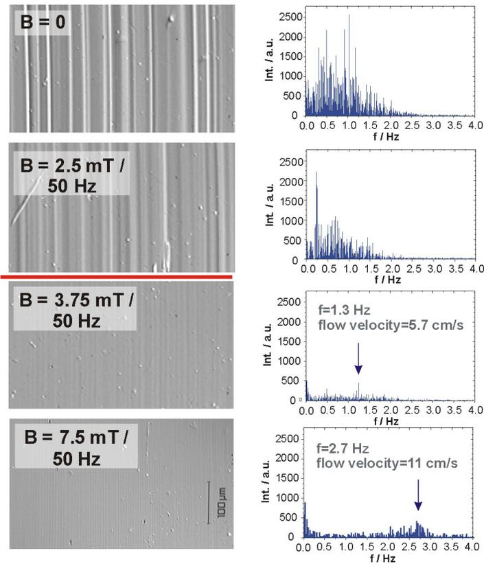
Fig. 4: Striation patterns (left column) and corresponding frequency distribution (right column) of an antimony doped silicon crystal grown under different rotating magnetic field strengths. The most significant change in the intensity of the dopant non-uniformities was found between 2.5 and 3.75 mT / 50 Hz (sample diameter: 14 mm) and shifts to higher values for smaller samples.
