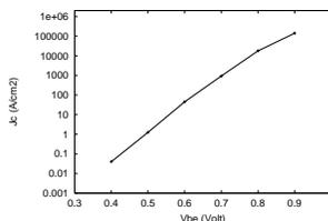
Figure 2: Collector current density for InP/InGaAs HBT
