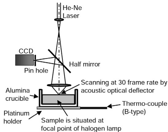
Figure 1: Schematic illustration of HLSCM system
