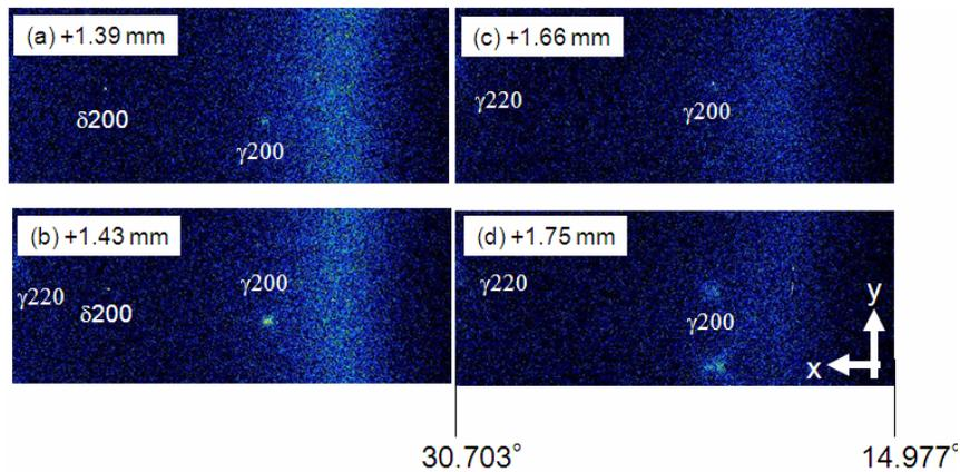
Figure 6: Diffraction pattern for peritectic reaction in solidification process of GTA welding
