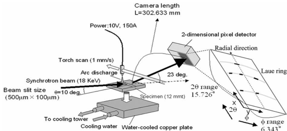
Figure 2: Schematic illustration of in-situ observation system in welding
