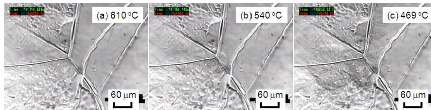
Figure 3: Perlite precipitation at the triple point and grain boundary of austenite
