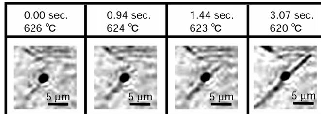
Figure 4: Acicular ferrite nucleated from oxide within austenite grain
