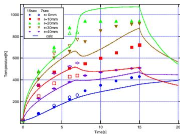
Figure 6: Measured and calculated plate temperature during spot heating test.
