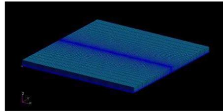
Figure 11: 3-dim. FE mesh used in the line-heating analysis.
