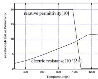
Figure 2: Temperature dependency of the electro magnetic properties.
