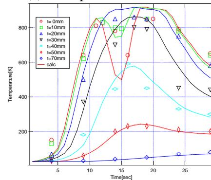
Figure 12: Comparisons of the measured and calculated plate temperatures during line heating tests.
