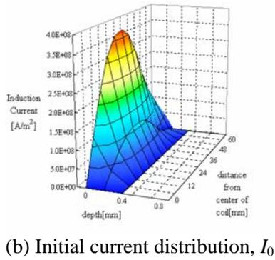
Figure 9:  $I_0$  and  $w$  identified from the spot heating test.
