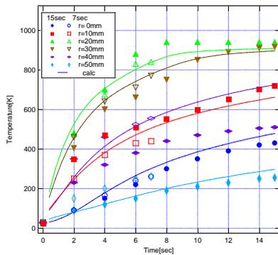
Figure 10: Comparison of the estimated plate temperatures calculated from the identified  $I_0(r,z)$  and  $w(T)$  with the measured ones.
