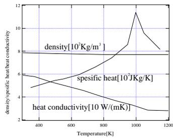
Figure 3: Temperature dependency of the thermal properties.
