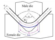
Figure 1: The bending process of metallic sheet (seated)
