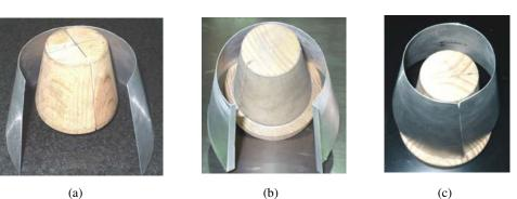
WTC #1: Dm = 70 mm ATC: Dm = 120.5 mm
