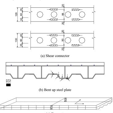
(c) Concrete Figure 1: Attachment positions of strain gauge
