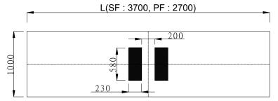
Figure 2: Position of load application
