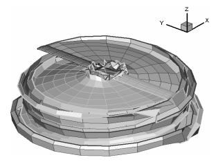
Figure 6: Wake geometry of 2-blade in the hovering
