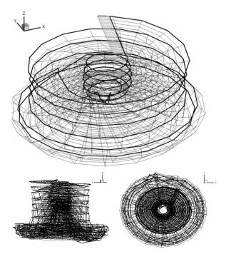
Figure 4: Wake geometry in the hovering with 1-blade
