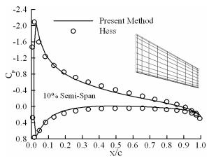
Figure 3: Pressure distribution of the thin swept blade
