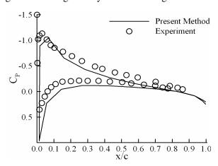
Figure 5: Pressure distribution of the 1-blade in the hovering
