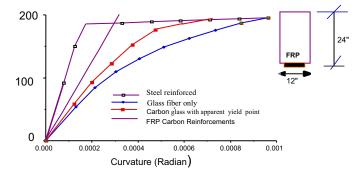
Figure 2: Moment Curvature Behavior of Fiber Material
