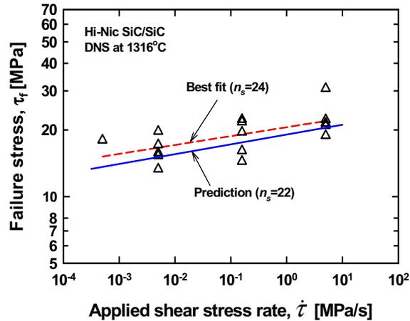
Figure 3: Comparison in interlaminar shear strength between the predicted and the actual data for Hi-Nic SiC/SiC composite in interlaminar shear tested at 1316 °C in air.
