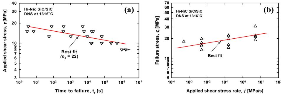
Figure 1: Results of (a) stress rupture testing and (b) constant stress-rate testing for Hi-Nic SiC/SiC composite in interlaminar shear (double notch shear, DNS) at 1316 °C in air. The solid lines represent the best fit.
