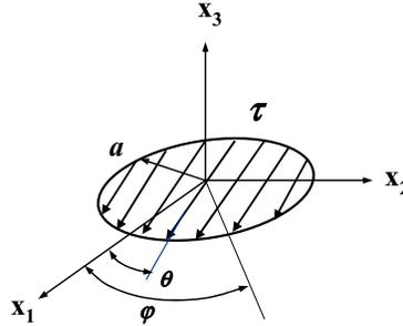
Figure 2: An assumed penny-shaped crack arbitrarily located at fiber-matrix interfaces in ceramic matrix composites, subjected to equal and opposite interlaminar shear stresses  $\tau$  acting on both surfaces of a crack.
