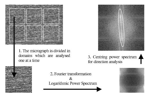
Figure 1: The three operations used to obtain a centred logarithmic power spectrum from a squared micrograph domain.
