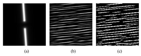
Figure 2: (a) Domain specific Fourier filter. (b) Result of inverse Fourier transformation after Fourier filtering. (c) Binary image obtained with a threshold value and thereby isolating individual fibres as elongated objects.
