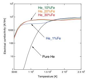
Figure 1: Dependence of electrical conductivities of helium gas on temperature for each mixing ratio.
