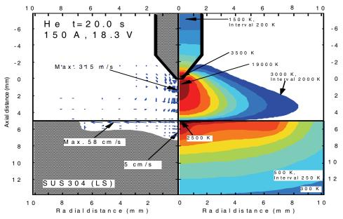
Figure 2: Calculated results for helium TIG arc welding for 150 A at 20 s after arc ignition.
