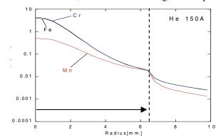
Figure 4: Concentrations of metal vapors around the anode surface.
