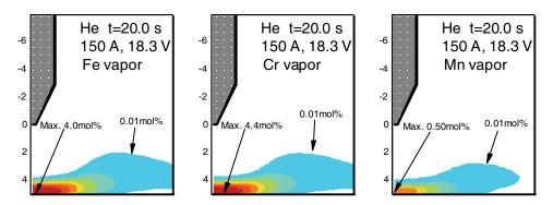
Figure 3: Distributions of iron, chromium and manganese vapor in arc plasma.
