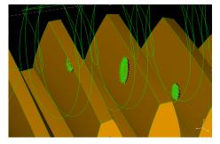
Figure 1: Load shared by gear tooth in contact
