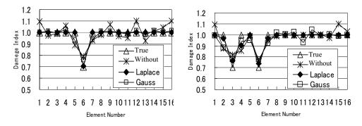
Figure 3: Damage detection of one damaged points model
