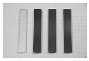
Figure 1: Inject-molded specimens (Neat PLA, 1wt%, 5wt%, 10wt%)
