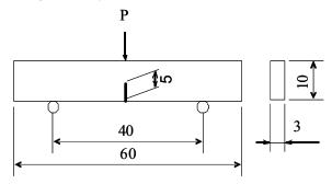
Figure 4: Fracture toughness specimen
