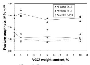
Figure 5: Fracture toughness
