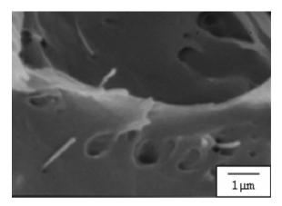
Figure 6: Fracture surface of amorphous composite specimen (10wt%)
