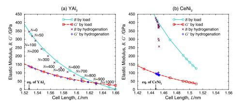
Figure 4: Elastic stability under isotropic tensile loading or by hydrogenation. N is the number of hydrogen atoms incorporated into  $A_{64}B_{128}$  systems. As for CeNi<sub>2</sub>, N < 37.
