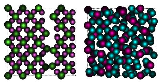
Figure 1: MD result of the fracture by isotropic tensile load. YAl<sub>2</sub> (left) shows cleavage fracture, while CeNi<sub>2</sub> (right) is collapsed to a amorphous-like structure.
