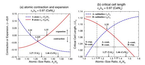
Figure 3: (a) Atomic contraction/expansion and (b) the critical cell length at the bulk modulus instability by the isotropic tensile load.  $\varepsilon$  is the Lennard-Jones energy parameter. R is the Goldschmidt radius of pure crystal state estimated by our potential. r is the radius in Laves phase.  $L_0$  is the equilibrium cell length at zero pressure. The ratio of energy parameters  $\varepsilon$  is adjusted for CeNi<sub>2</sub> while that of the size parameters are varied.
