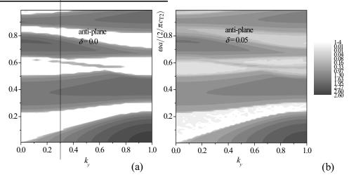
Figure 4: Localization factors and band structures vary with the normalized frequency and normalized wave number along the *y*-axis for the anti-plane wave propagating in crystals. (a) is for the ordered phononic crystal and (b) is for the disordered one with the disordered degree is 0.05.
