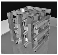
Figure 1: Artist's view of a 3D photonic metamaterial composed of elongated splitring resonators made by DLW of a polymeric backbone and subsequent coating via metal CVD.
