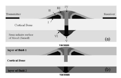
Figure 1: 2-D model of a healing bone in which the callus tissue consists of six ossification regions (denoted by capital Latin numbers). (a) The bone is immersed in blood, and (b) two layers of fluids load the upper and lower surfaces of the bone.
