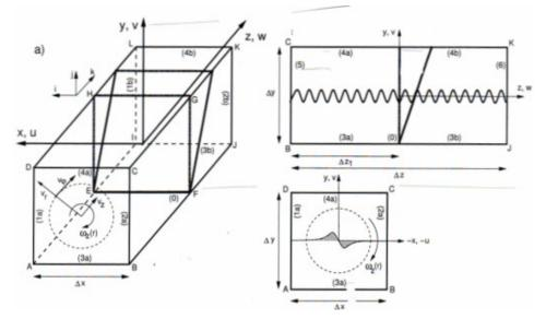
Figure 3: Computational domain for simulation of oblique- and normal-shock-vortex intersection, with initial position of shocks and vortex indicated [6].
