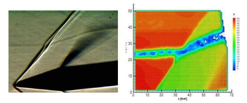
Figure 2: Intersection of a slender longitudinal vortex by an oblique shock at a Mach number Ma = 2.2, angle of attack of wing  $\alpha_w = 6^\circ$ , and of the shock generator  $\beta_s = 21^\circ$ ; standard schlieren visualization on the left, particle-image-velocimetry results on the right, pictures were taken from [5].
