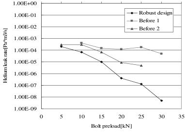
Figure 5: Results of helium leak test
