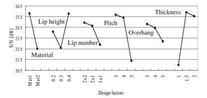
Figure 3: S/N plot: Contact area as evaluation criterion
