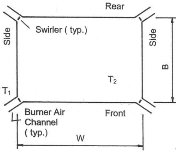
Fig. 1 Plan view of furnace with burners located in furnace corners ( schematic )
