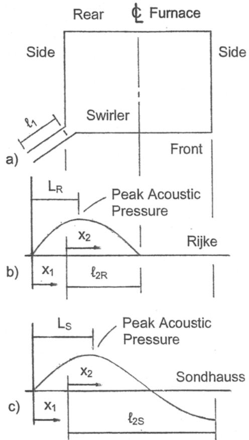
Fig. 3 Composite sketch of burner / furnace system with superimposed Rijke or Sondhauss acoustic pressure waves ( shown acoustic waves in furnace side-to-side direction )
