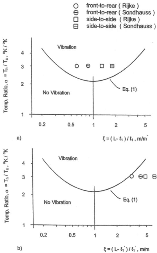
Fig. 4 Thermoacoustic stability diagram with superimposed evaluated data based on Rijke and Sondhauss thermoacoustic models a) original system with  $l_1 = 1.69\text{m}$  and b) modified system with  $l_1' = 0.61\text{m}$
