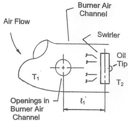
Fig. 5 Modified burner air channel showing openings to reduce original acoustic length  $l_1$  to new acoustic length  $l_1'$
