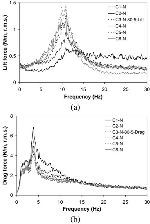
Figure 4: Typical dynamic lift and drag force spectra for 80% void fraction at 5 m/s pitch flow velocity: (a) Lift force spectra and (b) Drag force spectra
