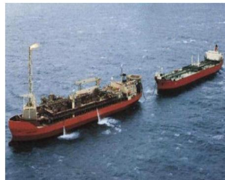
Figure 1. FPSO offloading operation
