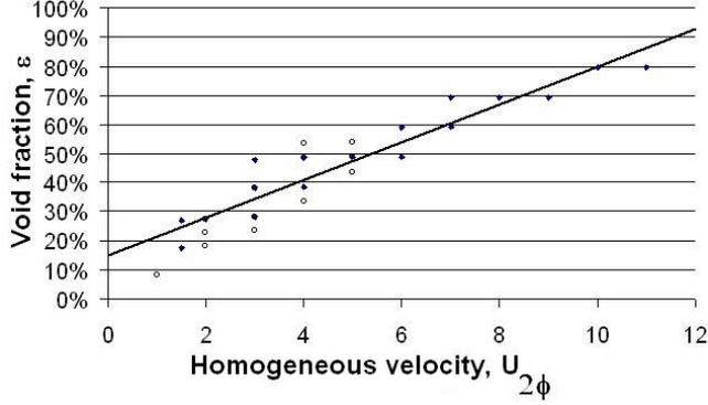
Figure 4: Void fraction ( $\varepsilon$ ) at maximum damping ratio with respect to homogeneous flow velocity. Diamond : Anscutter et al. (2006); circle : Present data
