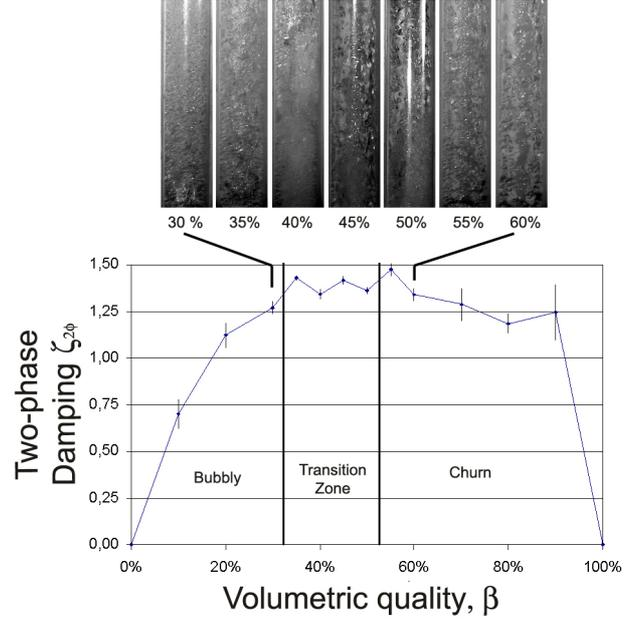
Figure 6: Two phase damping vs. Volumetric quality for  $U_{2\phi} = 4m/s$  and  $D_i = 13.4mm$
