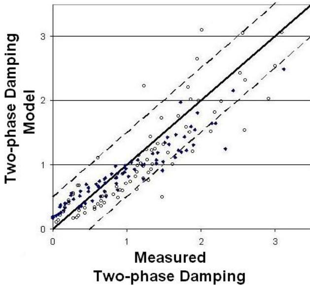
Figure 7: *Two-phase damping model vs measured two-phase damping. Diamond : Anscutter et al. (2006); circle : Present data*
