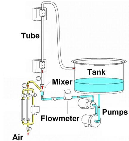
Figure 2: Test section
