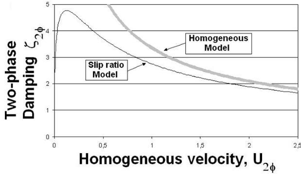
Figure 5: Two phase damping ratio vs. homogeneous flow velocity for  $\beta = 15\%$ . Thick gray line : homogeneous model ; thin black line : slip ratio model
